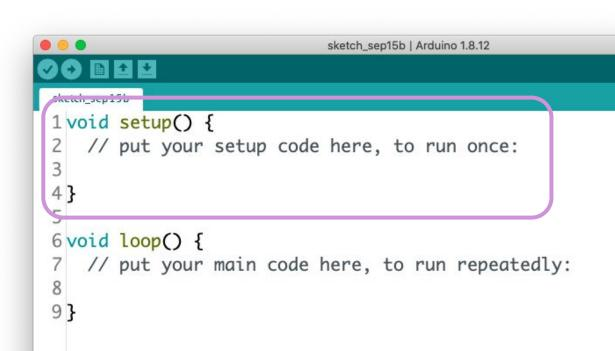
This code is run on initial start up of the Arduino. It's like the pre-flight checklist. It will run once.
